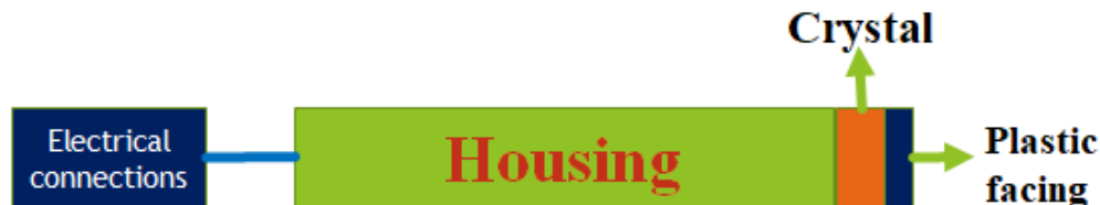
Figure 4 components of ultrasound transducer that produce ultrasound waves. The transducer probe consists of the piezoelectric disc with electrodes, electrical connections, the housing, and front facing.
